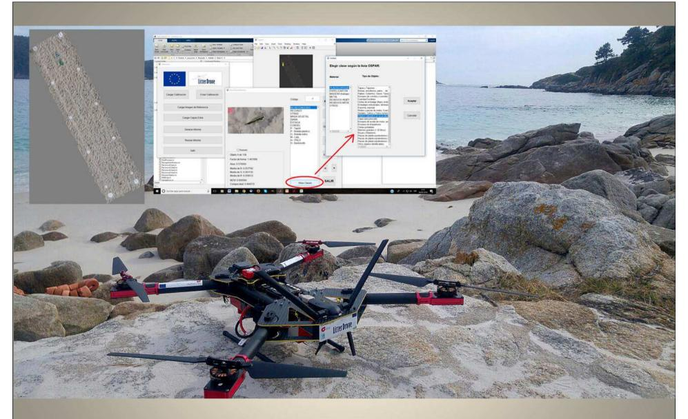
Drone-based image acquistion + Computer based image analysis.
